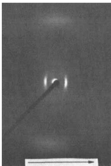
FIGURE 3 Flat camera picture of PCB 4, smectic A phase, fiber, arrow indicates drawing direction.
