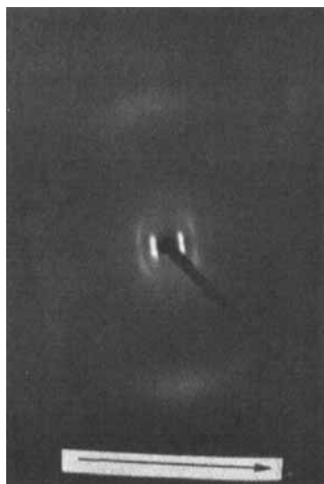
FIGURE 4 Flat camera picture of PCA 11, smectic C phase, fiber, arrow indicates drawing direction.
